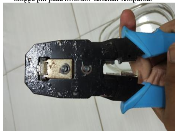
Gambar 7. Proses Crimping kabel
